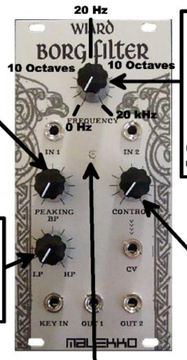
INITIAL CENTER FREQUENCY 0 TO 20khZ 20 OCTAVES Note: Half of knob travel from 0 Hz to 20Hz may not appear to be "working". It is working fine in the infrasonic range. Pleaase do not use near elephants (seriously)
