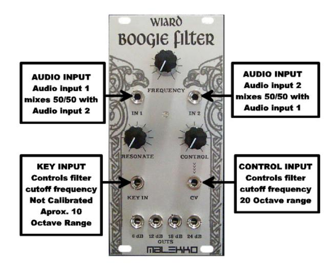
HINT: Route AD envelope to "KEY IN" route AR envelope to "CONTROL IN" for simple ADSR mixer. Use "CONTROL IN" as simple "SUSTAIN" control. Use initial frequency for "PUNCH" "Thanks to John Paia Simonton for suggesting "PUNCH" mode RIP."
