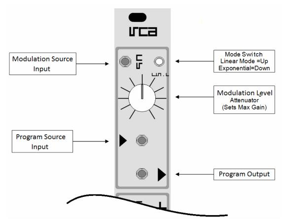
**Modulation Source Input:** When either an audio or control signal is routed from the Program Source Input to the Program Output jack, the signal applied to the Modulation Source Input jack controls the program level (if audio, "Volume"). Typical Modulation sources are LFO's, Envelopes, and foot pedal controllers.
