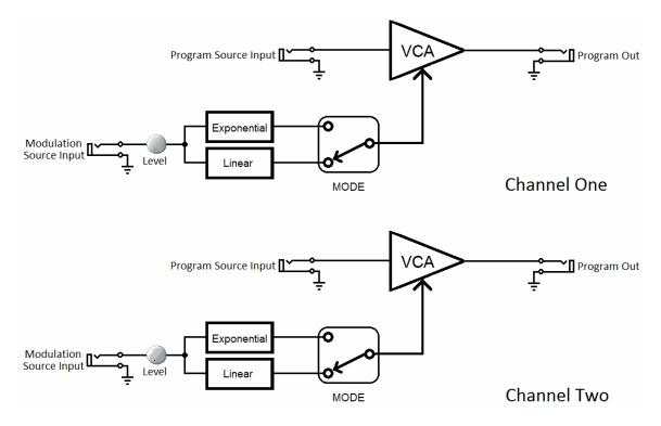
**Linear and Exponential Modes:** The front panel mode control switch selects Linear modulation response when in the fully "up" position and Exponential response mode when depressed.
