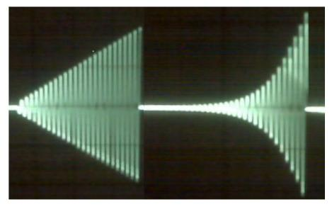
In practice this means an envelope contour that slowly changes volume when in Linear mode, quickly produce a more quick volume change in Exponential mode.
