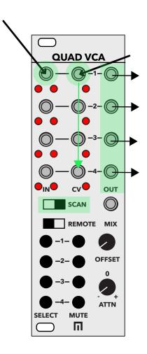
PAN - Insert an input into Ch. 1 and Ch. 1 CV will route input to up to 4 different outputs.
