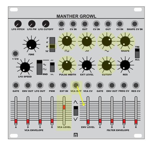
Turn up the VCF Filter cutoff control per diagram, set the manual controls for the Square, Saw, and Tri-Shape controls. Dial the Pulse Width control to 12 o'clock. Sweep the SHAPE (waveshape) control left to right.
