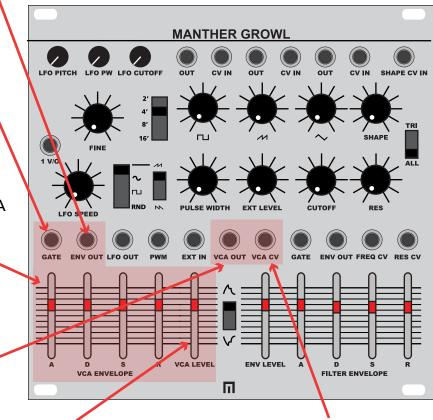
VCA CV INPUT: CV input controls VCA level. Accepts 0 to +5V.
