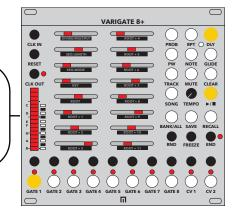
To clear an existing pattern, simply hold the CLEAR button while selecting one of the GATE buttons to clear that pattern/sequence entirely.
