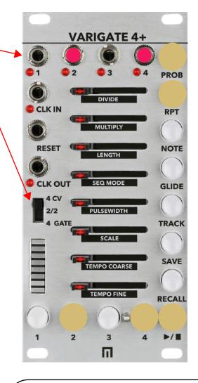
**COPY/PASTE**: To copy and paste newly programmed step sequence data to another channel, simply hold down one of the CHANNEL buttons while selecting another channel button.
