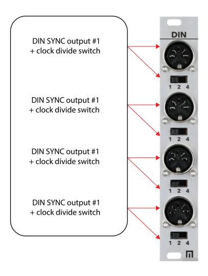
**DIN SYNC**: Incoming CLOCK from your computer or external device (connected to the Malekko Sync module) will output to the DIN SYNC outputs. Each output can be divided up to 4 times.
