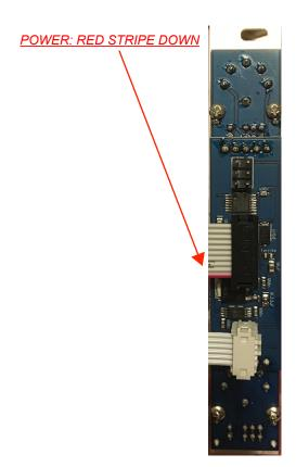
6-PIN CONNECTION TO MALEKKO SYNC (IF YOU ARE ONLY USING DIN SYNC WITH SYNC IGNORE THE CV GATE CONNECTION)
