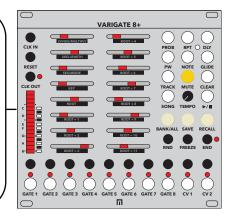
**COPY PATTERN**: To copy a pattern from one channel to another, hold the source channel and press the destination channel.
