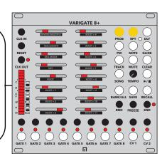
**FREEZE**: This gate input is active high. Inserting an external gate will freeze randomization. You can also FREEZE by *holding* down the RECALL button for 2 seconds and it will flash and stay held until you press it again for 2 seconds.
